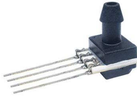
Figure 9: Absolute pressure sensor used in the lab [8].
